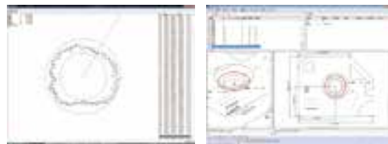
Drawing the geometrical deviation of a circle Graphical display of a measured element
