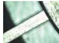
Positive edge detection with co-axial light
