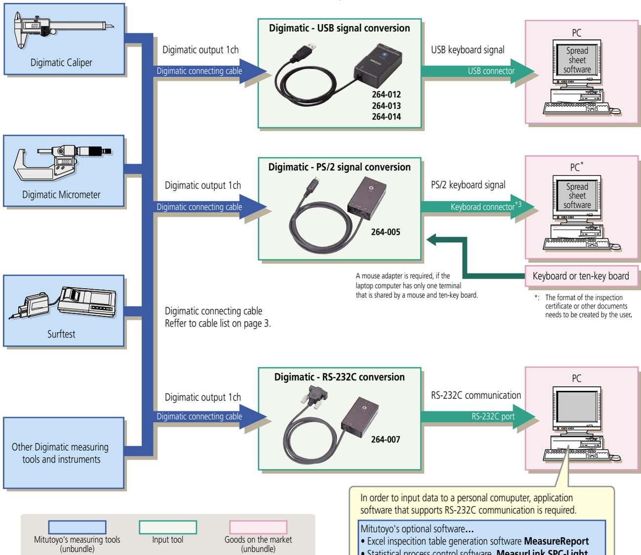
In order to input data to a personal computer, application software that supports RS-232C communication is required.
