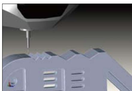
Creating nominal sections from CAD data (CAT1000S)
