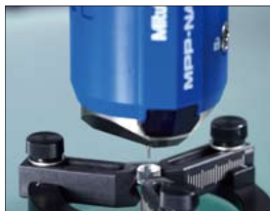
Aspheric-form MPP-NANO measurement
